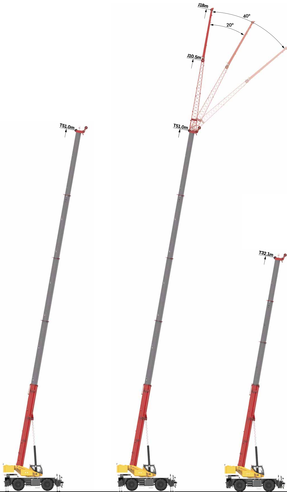
Telescopic boom on outriggers 主臂、支腿吊载
