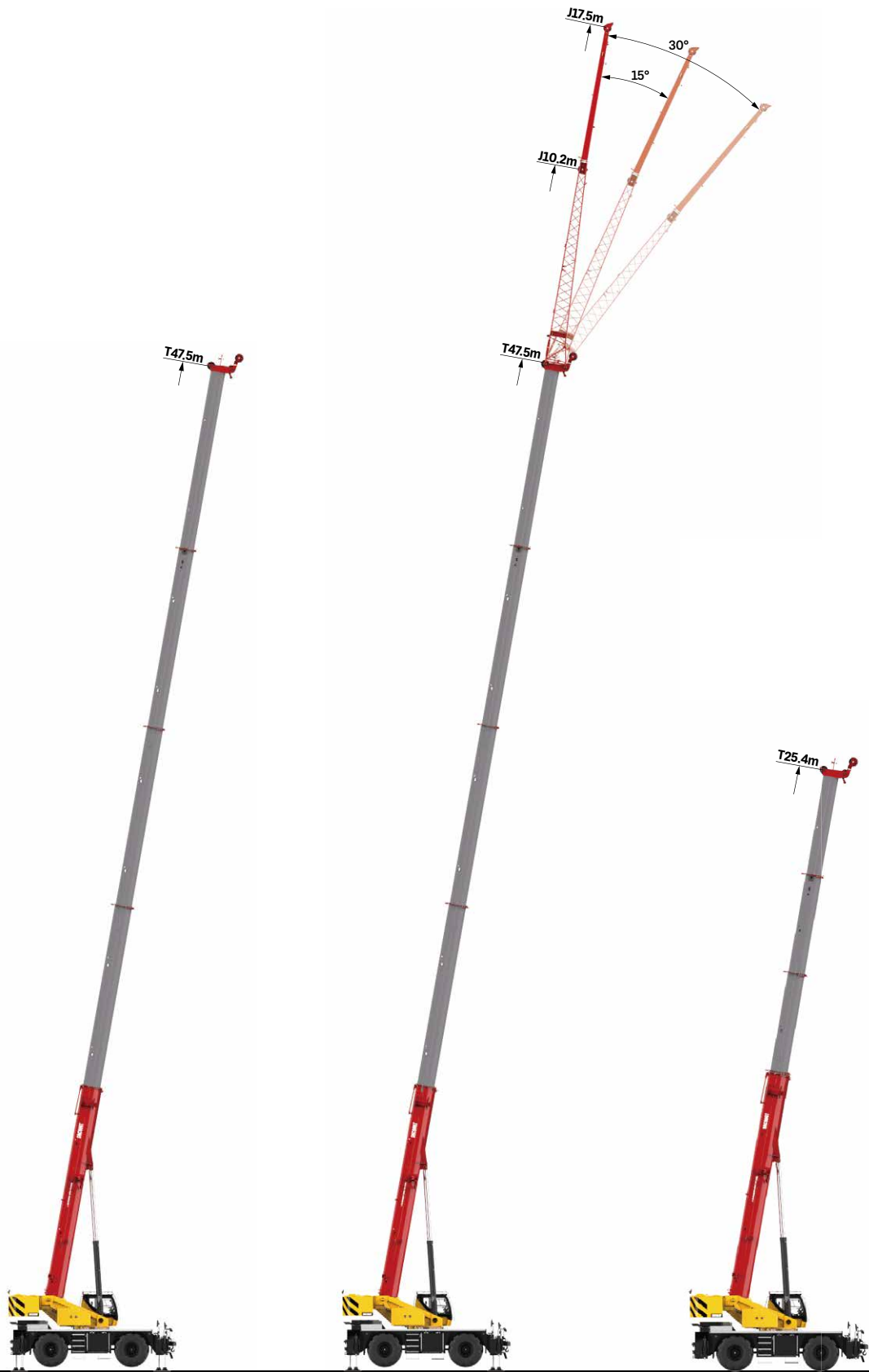
Telescopic boom on outriggers 主臂、支腿吊载
